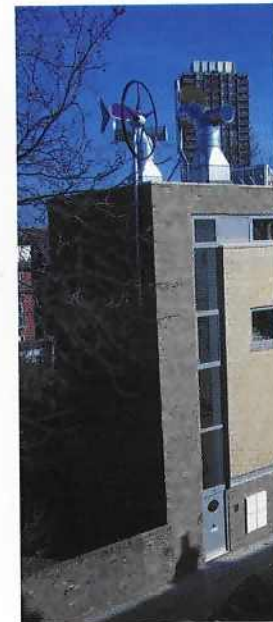
New developments in technology allow small wind turbines to be quiet enough to be building mounted
