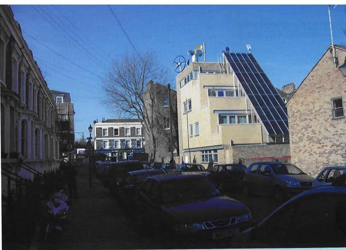
New developments in technology allow small wind turbines to be quiet enough to be building mounted
