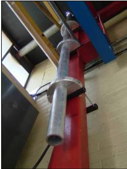
Figure 25. Swift turbine mounting pole (fixed internally)
