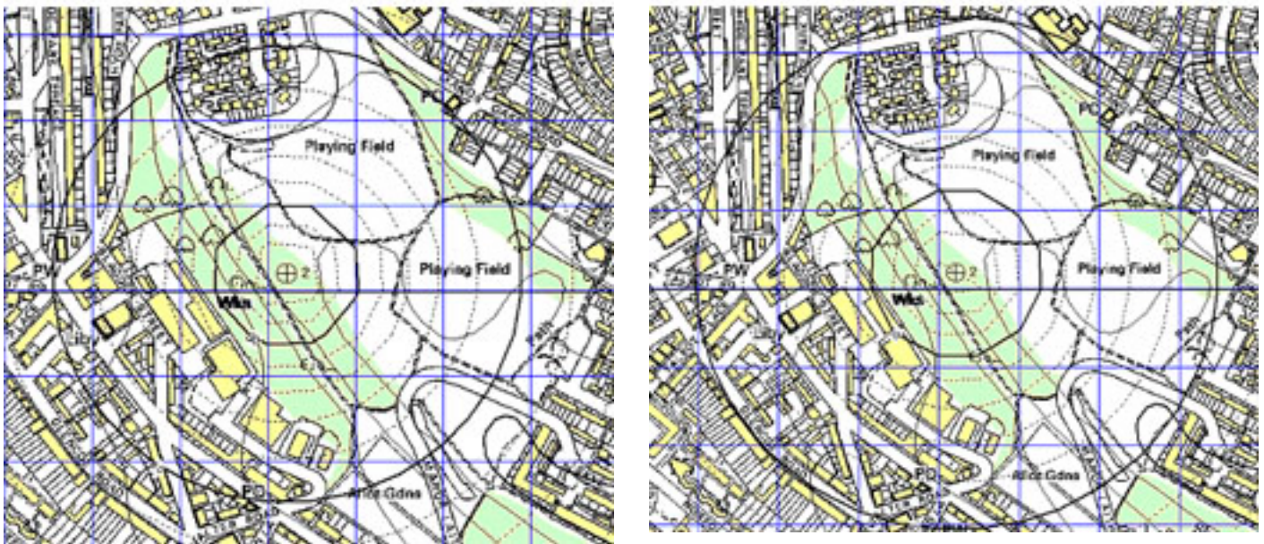
Figure 45. Noise profile for a 300kW and a 600kW wind turbine
