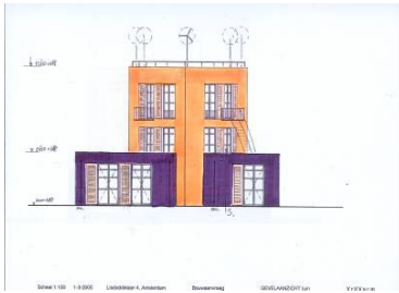
Figure 6: Draft of the house with 5 urban turbines
